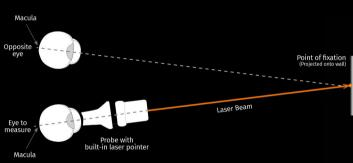
ProBeam™ is exclusive to Quantel Medical. The probe generates a laser beam that creates a focal point for the patient to look at: this facilitates measurement while increasing the precision of the probe<sup>2</sup>.
